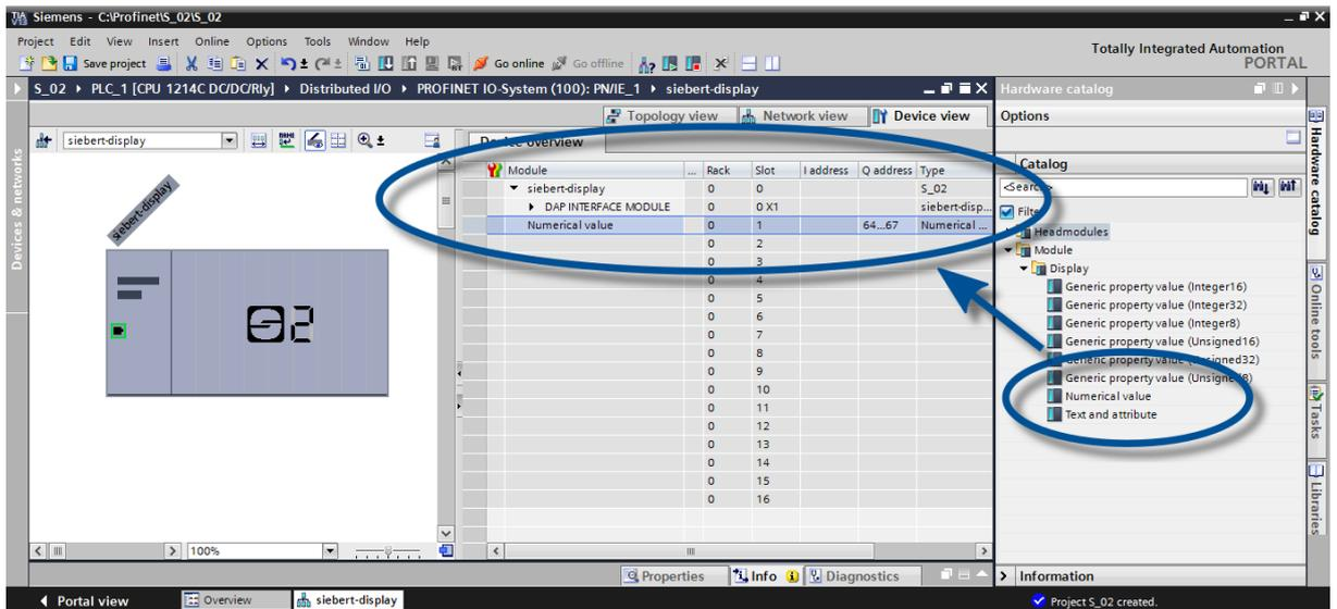
The screenshot shows the 'Hardware catalog' and 'Device overview' in Siemens TIA Portal. The 'Device overview' table lists modules for the 'siebert-display' rack. A blue circle highlights the 'Numerical value' module in slot 1, which is assigned to I address 64 and Q address 67. The 'Hardware catalog' on the right shows the 'Numerical value' module selected under the 'Display' category.
